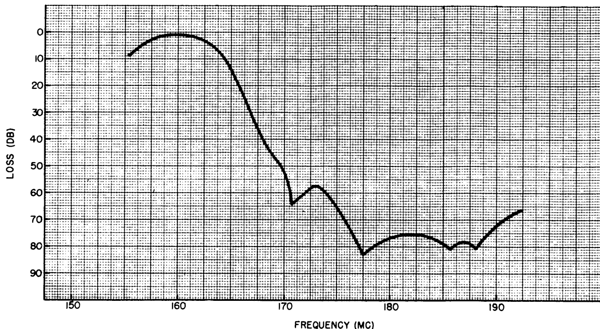
Figure 6-20. 163 Mc Low Pass Filter, Response Curve
