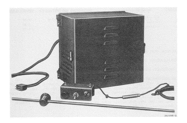
Radio Receiving Set AN/VRR-2 is a vehicular, single fixed-frequency, a-m (voice), medium range, receiving equipment used in traffic control, monitoring, and similar applications by military police, guard, and security troops.
