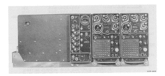
Radio Set SCR-808 is a vehicular, crystal-controlled, short-range, f-m (voice only) radiotelephone equipment used for coast artillery, military police, security, and similar operations.
