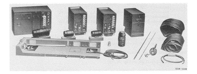
Radio Set SCR-508 is a vehicular, medium-range, crystal-controlled, f-m (voice) radiotelephone equipment used by armored units.
