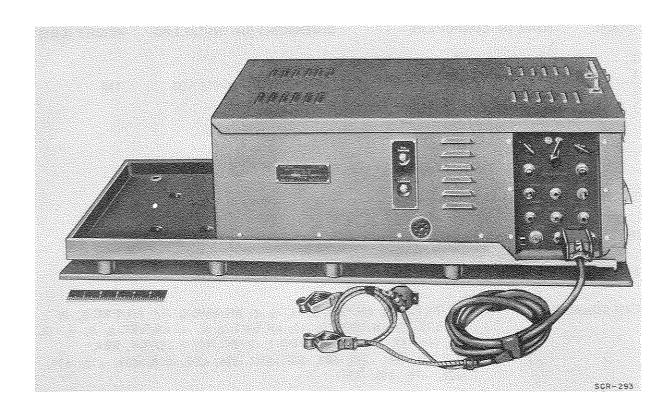
Radio Set SCR-293 is a vehicular short-range, medium-power, f-m (voice) equipment used in inclosed vehicles for two-way voice communication within and between armored units or between armored and infantry units.
