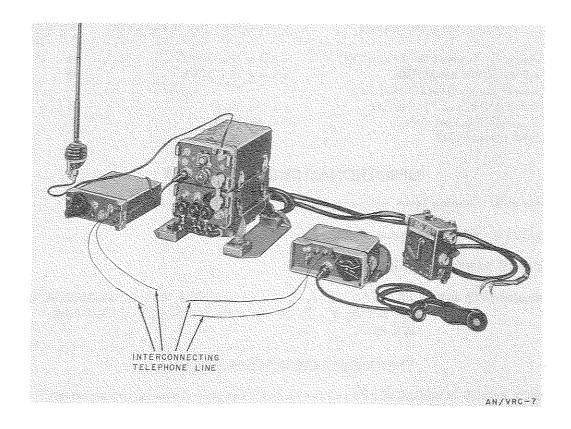
Radio Set AN/VRC-7 is a short-range, f-m (voice), vehicular radiotelephone equipment used within and between artillery, infantry, and armored force units.
