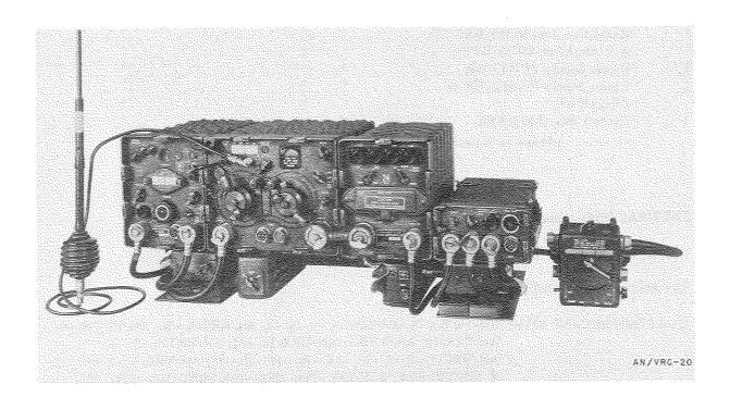
Radio Set AN/VRC-20 is a vehicular, short-range, f-m (voice), radiotelephone equipment for communication within and between armored units and for liaison between armored and artillery units.
