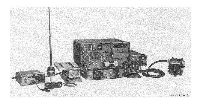
Radio Set AN/VRC-13 is a short-range, vehicular, f-m (voice) equipment for communication within and between armored units and for liaison between armored force and artillery units.
