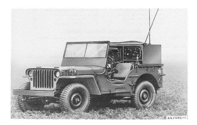
Radio Set AN/VRC-1 is a short range, h-f and v-h-f, a-m (voice, tone, and cw) radio transmitting and receiving equipment which may be installed in vehicles for ground-to-air communication at Air Force bases and similar installations.
