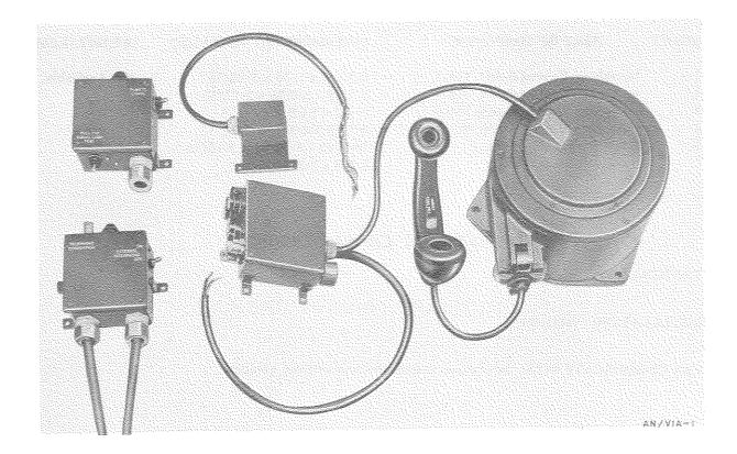
Auxiliary Interphone Equipment AN/VIA-1 is an assemblage of auxiliary components used to extend a vehicular interphone system to the exterior of the vehicle. It is used in inclosed or armored vehicles.
