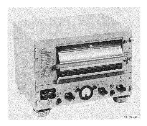
Facsimile Recorder RD-92/UX is used to make direct recordings of copy transmitted by Facsimile Transceiver TT-41/TXC-1B. It may be used for recording facsimile signals from either wire or radio communication circuits.
