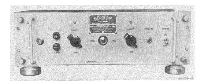
Radio Modulator MD-168/UX is a subcarrier frequency-shift unit operating on frequencies of 1.5 to 10 kc. It converts amplitude-modulated facsimile signals to audio frequency-shift signals of constant amplitude, which in turn are used to modulate the carrier of a radio transmitter.
