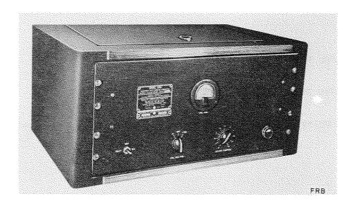
Frequency Shift Receiver Equipment FRB is used for the demodulation of facsimile or radio-photo frequency-shift signals, and is used aboard ship or at shore stations.
