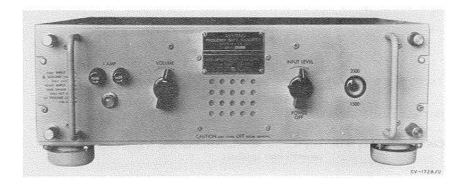
Frequency Shift ConverterCV-172A/U converts1,500-2,300 cps facsimile signals (received from a radio circuit) to a-m signals for a facsimile recorder. The signals from the radio receiver are audio frequency shift signals in which 1,500 cps represents black and 2,300 cps represents white for the recorder.
