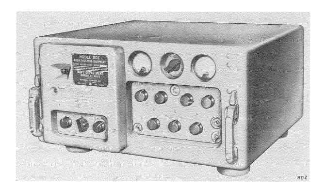
VHF Radio Receiving Equipment RDZ is a general purpose, crystal-controlled, radiotelephone receiver which operates in the v-h-f/u-h-f range of 225 to 400 mc.
