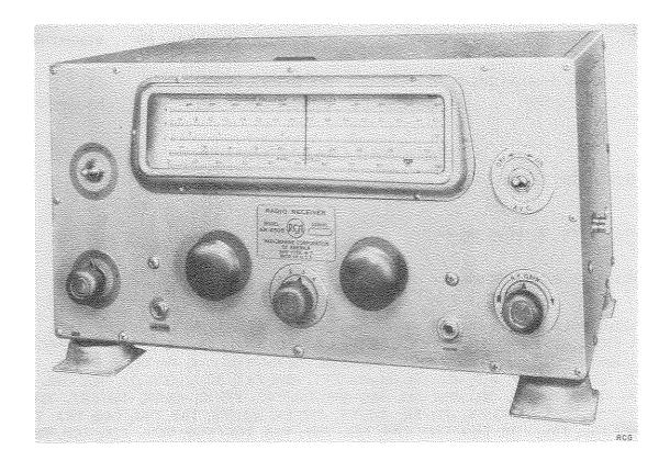
Radio Receiving Equipment RCG is an a-c/d-c general purpose receiver of radiotelegraph or radiotelephone signals within the m-f and h-f ranges.
