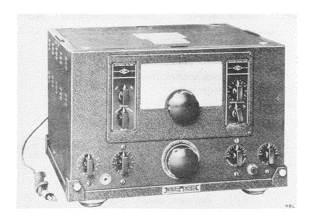
Radio Receiving Equipments RBL, RBL-1 and RBL-2 are general purpose, tuned r-f receivers of telegraph signals between 0.015 to 0.6 mc. Voice reception is only possible above 0.2 mc. The level of r-f radiations is kept below 400 uuw making their use safe within combat areas.
