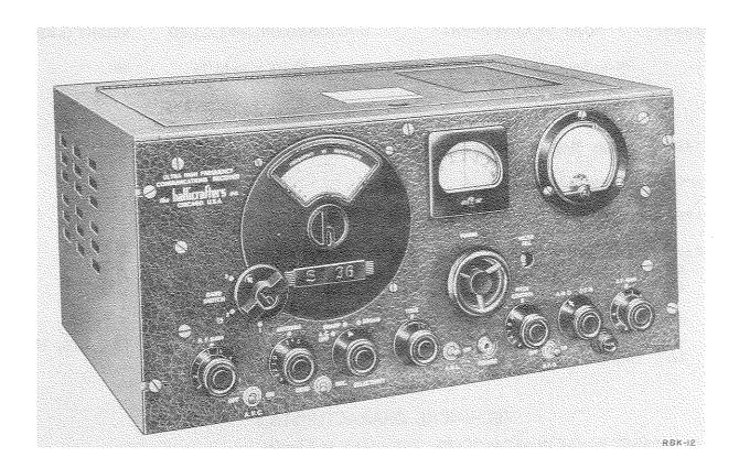
Radio Receiving Equipments RBK-12 and RBK-13 are general purpose, v-h-f (am or fm) radio receivers of radiotelephone or radiotelegraph signals and can also be used with a panoramic reception adapter.
