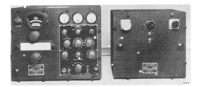
Radio Receiving Equipments RBC, RBC-1 through RBC-6 are general purpose, radiotelegraph, or radiotelephone receivers operating within the frequency band 4.0 to 27.0 mc.
