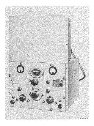
Radio Receiving Equipment RBA-6 is a general purpose, tuned r-f receiver used for shipboard or shore station radio reception in the low- and medium-frequency bands.
