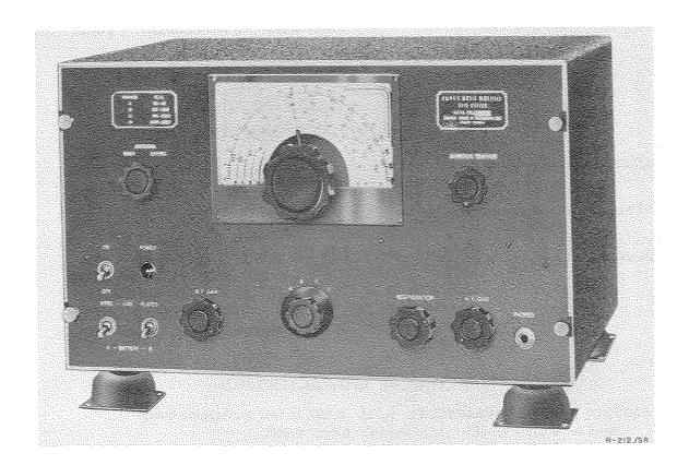
Radio Receiver R-212/SR is a tuned-radio-frequency, a-m (cw, icw, and mcw) radiotelegraph receiving equipment used in shipborne and fixed station applications.
