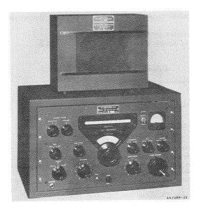
Radio Receiving Set AN/URR-23 is an a-m (cw, mcw, and voice) equipment designed for general purpose communication applications which require the highest order of stability and dial accuracy. It is suitable for a-m and c-w reception or for presetting at a specific frequency without repeated search or frequency readjustment.
