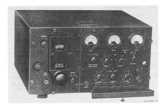
Radio Receiving Sets AN/URR-21 and -21A are a-m (voice) v-h-f receivers used in conjunction with VHF Radio Transmitting Equipment TDQ on aircraft carriers, and at shore stations, for communicating with aircraft.
