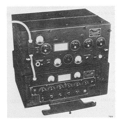
VHF Radio Transmitting and Receiving Equipments TBS and TBS-1 through -8 provide a-m (cw, voice) radio communication between surface craft, and between submarines and surface craft. They are crystal-controlled and provide for full control of the transmitter from remote positions.
