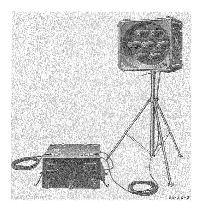
Public Address Set AN/UIQ-3 is a transportable, high-power, long-range, sound amplifying and projecting equipment used for directing landings, commanding ground operations, issuing orders under combat conditions, and similar operations.
