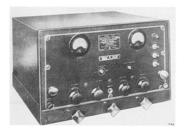
Frequency Shift Receiver Converter Equipment FRA is a single channel, i-f type set for translating radiotelegraph characters and furnishing d-c mark-and-space pulses for operation of a teletypewriter when used in conjunction with Radio Receiving Equipments RBB and RBC.
