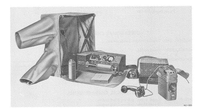
Facsimile Equipment RC-120 is a transmitting and receiving set used for communicating graphic copy. It will receive positive and negative photographs, printed or written copy, and similar material on film or direct on teledeltos paper which requires no processing. It is used in fixed stations over communication circuits serving corps and higher headquarters.
