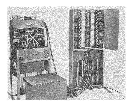
Telephone Central Office Set TC-4 is a complete, transportable, field telephone exchange for handling magneto line traffic, and for originating and terminating common battery trunk line and ring-down tie line traffic at division level.
