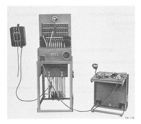
Telephone Central Office Set TC-12 is a complete, transportable or mobile, tactical telephone exchange for handling, originating, and terminating trunk and tie line traffic and is used in field wire and cable systems serving regimental and higher headquarters.
