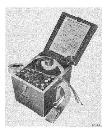
Telephone Repeater EE-89 is a portable, two-wire repeater equipment which is installed at intermediate points of a tactical field wire system (at junctions of sections having similar characteristics) to extend the normal transmission range of facilities serving division and higher headquarters.
