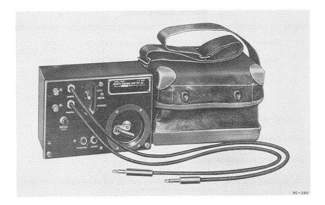
Remote Control Equipment RC-290 is an assemblage of items enabling the erection of a local battery telephone facility between a displaced operating and control position and the actual operating site of field radio equipment. It is used in conjunction with radio communication equipment organic to battalion level units.
