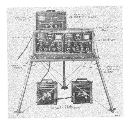
Portable Radio Receiving Equipments RBM-1, -2, and -3 are primarily intended for general purpose field service. They consist of two receivers which may be operated separately or together, permitting simultaneous reception on the m-f and h-f range.
