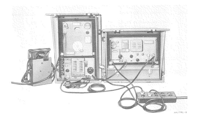
Radio Set AN/TRC-8 is a transportable, v-h-f, f-m, single-channel radio receiving and transmitting equipment used for point-to-point or radio relay applications at division or higher headquarters.
