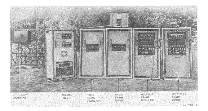
Radio Set AN/TRC-6 is a transportable, pulse-position-modulated, superhigh-frequency radio relay set used at terminals of a multichannel radio relay system in conjunction with v-f or carrier telegraph and telephone facilities. It is usually installed at permanent or semipermanent locations at higher head-quarters.
