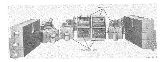
Radio Relay Set AN/TRC-4 is a transportable, crystal-controlled, f-m, field, radio transmitting and receiving equipment which can be used in point-to-point, single or multichannel communication or as the repeater facility of a radio relay link of a system serving corps and equivalent headquarters.
