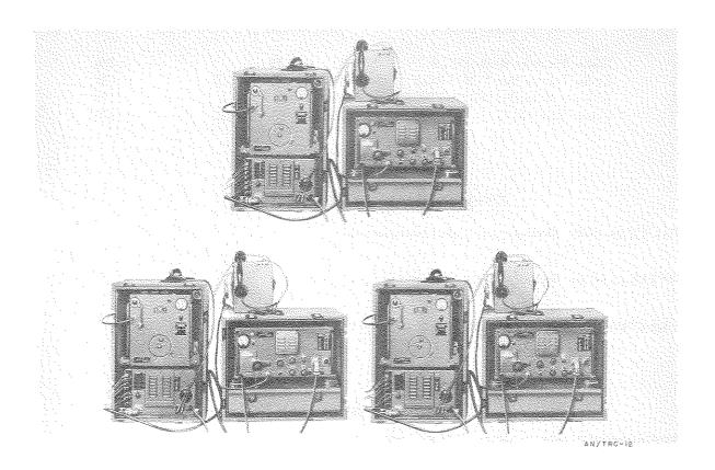
Radio Relay Set AN/TRC-12 is a transportable, f-m (voice), v-h-f transmitting and receiving equipment used for single-channel, point-to-point communication or as a repeater station at intermediate points of a radio relay system serving division and higher headquarters.
