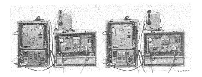
Radio Terminal Set AN/TRC-11 is a transportable, f-m (voice), v-h-f, transmitting and receiving equipment used for single-channel, point-to-point communication or as the terminal of a radio relay system serving division and higher headquarters.
