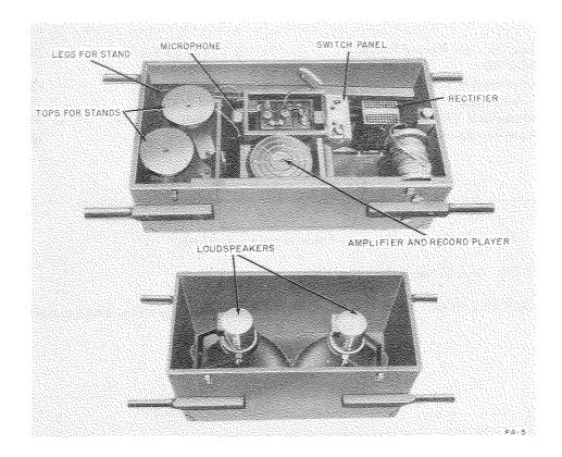
Public Address Set PA-5 is a portable public address or sound projecting equipment by means of which voice or music from a microphone or record input can be amplified and projected to audiences. It is used for delivering commands or for briefing in forward areas.
