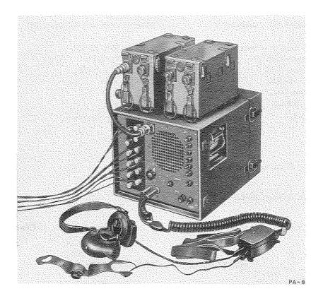
Intercommunication Set PA-8 is rugged, portable, sound-amplifying and projecting equipment used as a loudspeaker intercommunication system serving displaced elements of a field artillery battery.
