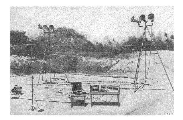
Public Address Set PA-2 is a transportable, medium-power, public address, or sound projecting equipment by means of which voice or music from a microphone, record player, or radio tuner can be amplified and projected to audiences. It is used for delivering commands, briefing, and training or for recreational and morale activities. It can be used on the ground, either indoors or outdoors.
