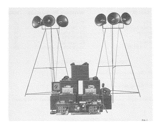
Public Address Set PA-1 is a transportable, medium-power sound amplifying and projecting equipment used in conjunction with microphone, record player, radio, or equivalent sound signal sources for commands, briefing instructions, training and morale applications, and similar uses at posts, camps, and stations.
