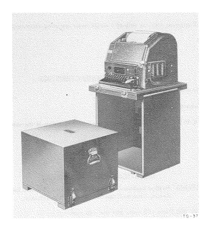
Teletypewriter TG-37 is a portable, field, page-printing, teletypewriter station equipment having weather communication keyboard and type-pallets, and is used at division and higher headquarters.
