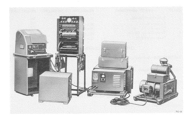
Telegraph Central Office Set TC-3 is a complete transportable central office for receiving, transmitting, and switching tactical teletypewriter traffic in a field wire or cable system serving division or higher headquarters.
