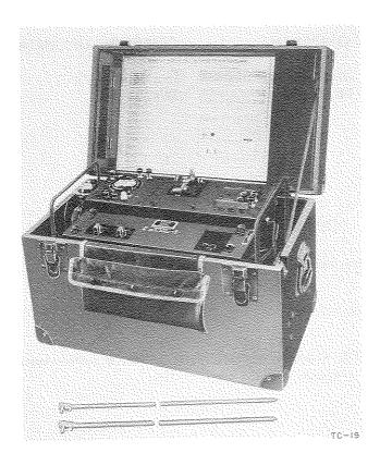
Repeater Set TC-19 is a portable, field, d-c telegraph repeater used for single operation at intermediate points between terminal repeater equipment in facilities serving division and higher head-quarters.
