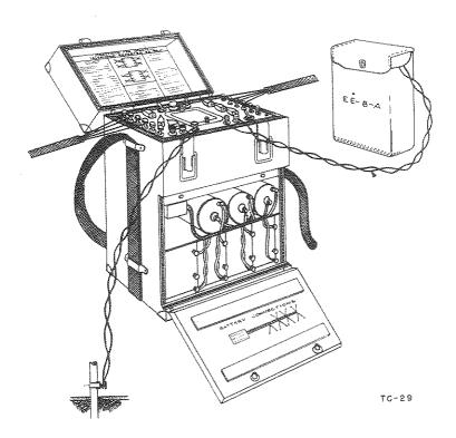
Telephone Repeater Set TC-29 is a portable repeating equipment used at intermediate or terminal points of a field telephone system to extend the transmission range of facilities serving division or higher headquarters.
