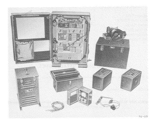
Repeater Set TC-23 is a transportable, four-wire, carrier repeater equipment used at intermediate points in a spiral-four cable carrier facility serving division and higher headquarters.
