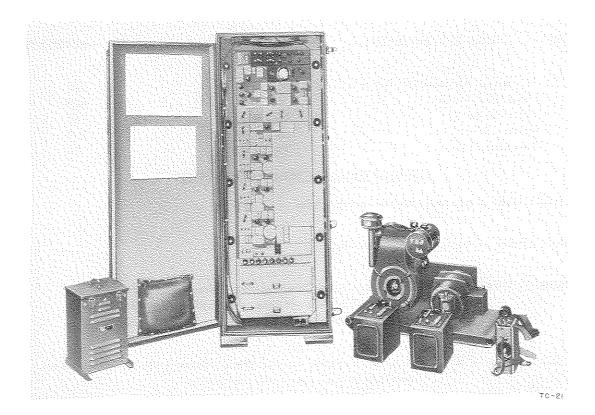
Telephone Terminal Set TC-21 is a carrier telephone terminal equipment which provides four v-f channels over a 100-mile spiral-four system, an open wire pair, or a combination of these facilities, for telephone and teletypewriter communication in long-range tactical carrier communication applications.
