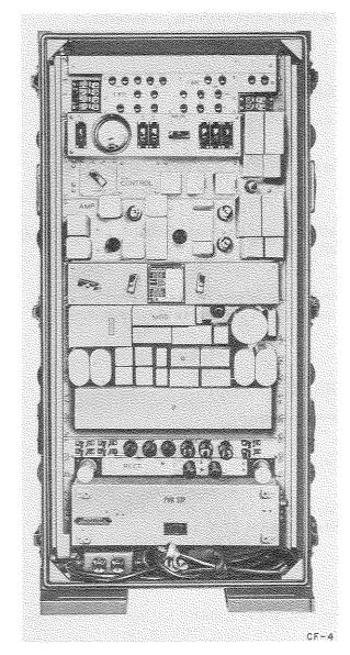
Converter CF-4 is carrier-converter equipment, designed to be used at junctions of open wire and Telephone Terminal CF-1, or spiral-four cable, to change four-wire operation from the terminal (or the cable) to effective two-wire operation over the open wire pair. It is used in systems serving corps or higher headquarters.
