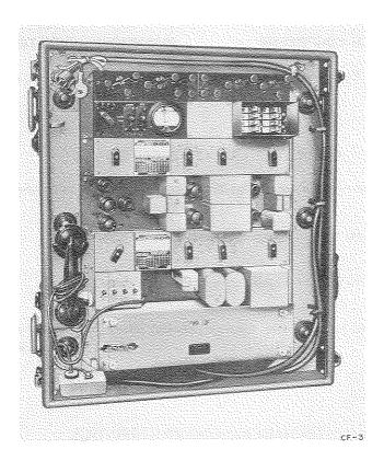
Repeater CF-3 is a carrier repeater equipment used to extend the range of telephone and telegraph carrier facilities using spiral-four or equivalent wire or cable in systems serving division, corps, or higher headquarters.
