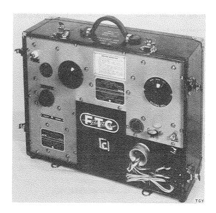
Portable Emergency Radio Transmitting Equipment TCY and TCY-1 are used for emergency or distress signaling by inexperienced personnel in lifeboats or liferafts. They radiate "SOS" or "SSS" signals on the international distress frequency of 0.5 mc.
